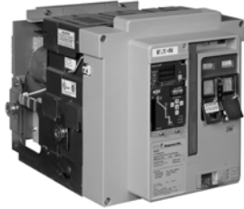
The Magnum MDSL current limiting power circuit breakers have integral current limiters to provide interruption ratings of 200 kA at 600 Vac.
