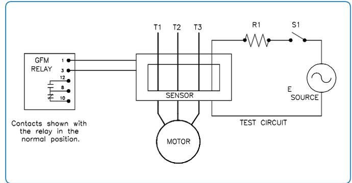
A Simulated fault current can be applied by the above test circuit. An appropriate value of R1 should be selected to apply a minimum of 1.5 times maximum trip rating of the sensor.
