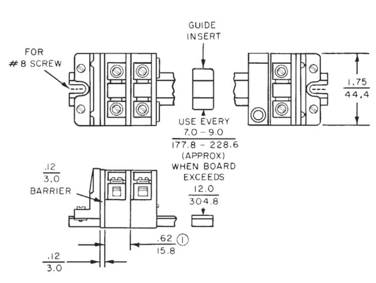
① On CR151A1 30-amp box terminals, width of block is .42 inches (10.7 mm).
